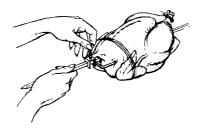
Finish securing food on spit by gliding second 2-pronged fork onto spit with prongs toward food. Tighten screws to a flat surface on spit.
